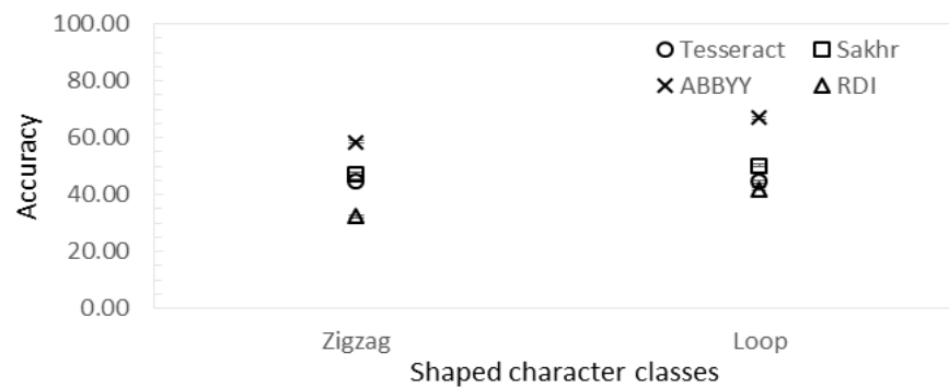
Figure 3.11. Character accuracy based on shaped character results from the OCR system evaluation
